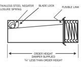
(H) HORIZONTAL MOUNT HORIZONTAL MOUNTING MODELS INCLUDES STAINLESS STEEL NEGATOR SPRINGS AND BLADE LOCKS
